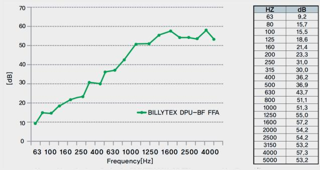
Measured Insertion Loss ILv for the BILLYTEX DPU-BF DC, expressed in dB per 1/3-octave frequency band. The insertion loss ILv refers to the mean velocity level in dB re  $10^{-9}$  m/s.
